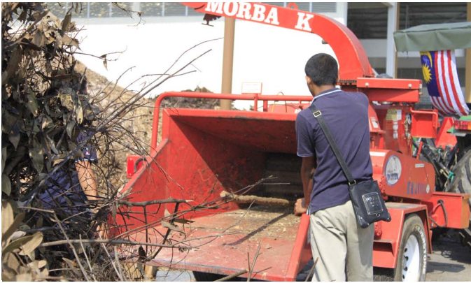
Tree trunks and branches has to be shredded before the composting process.
