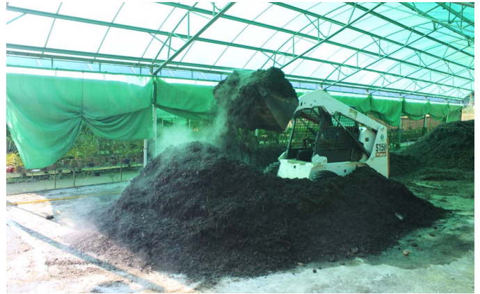
The process of turning the compost has to be carried out every three days for the purpose of aeration.
